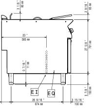
4 15/16 " 126 mm Electrical inlet (power) EI = EQ Equipotential screw
