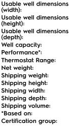
340 mm 575 mm 400 mm 21 It MIN; 23 It MAX 37.5 kg\hr 105 °C MIN; 185 °C MAX 57 kg 70 kg 1080 mm 460 mm 1020 mm 0.51 m<sup>3</sup> ASTM F1361-Deep fat fryers EFE91M23
